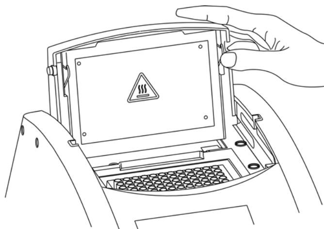
Figure 8. Rest the lid in vertical position
