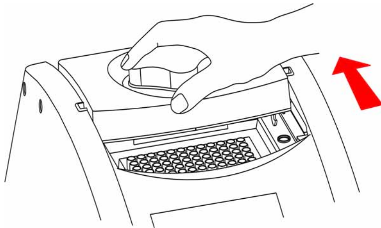
Figure 6. Slide the lid to align the lid hinge with notches of top case
